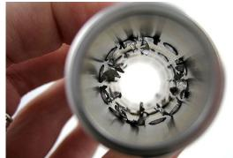
Cross-drilled holes act as conduits for fluids, lubricants and gases. Failing to remove burrs can cause blockage of these critical passages or create turbulence in the flow.
