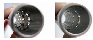
According to one machining expert, flexible hones are a cost-effective solution to smooth edges and produce a blended radius for crosshole deburring.
